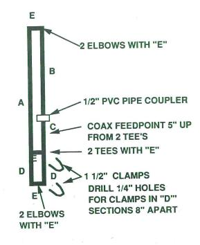
Recheck everything and when everything is straight, solder it all together. USE CAUTION AND CARE WHEN SOLDERING WITH A FLAME. BE CAREFUL AND DON'T TOUCH THE HOT COPPER PIPES.
